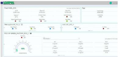
A reporting dashboard shows all the data collected by the IoT Air Quality Monitor sensors so that the plant end user can read it and continuously monitor a number of air pollutant parameters.
